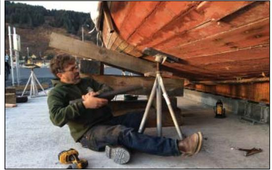
*Contractor shipwright Brian Johnson cribbing the Thelma C prior to installation of a permanent steel boat cradle.
